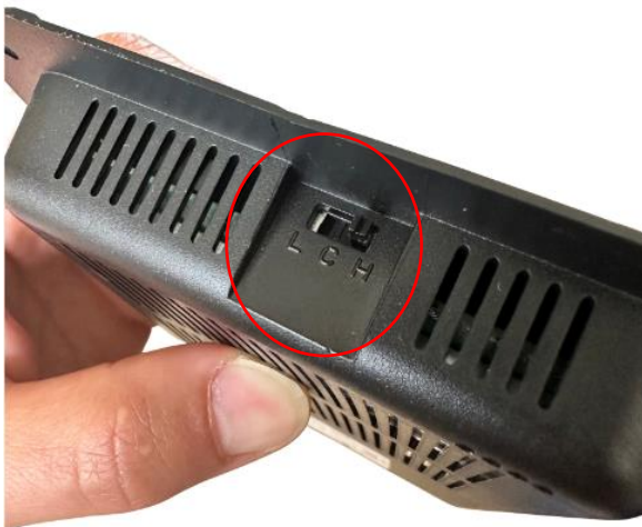
5. Set charger switch position according to thickness (H setting for 12mm)
