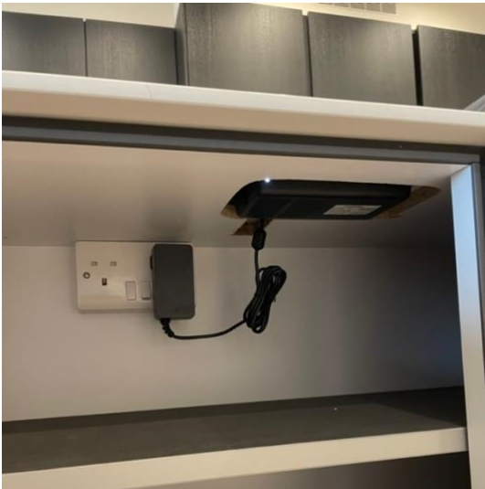
3. Mount charger using tape provided and plug in
